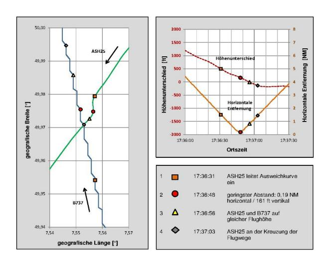
**Image 1:** Flight paths of the Boeing B737-800 and the powered glider Source: QAR/GPS data, analysis BFU
