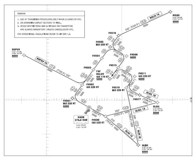
**Image 2:** GPS/FMS RNAV Arrival Chart Transition to Final Approach (Overlay to Radar Vector Pattern) RWY 21
