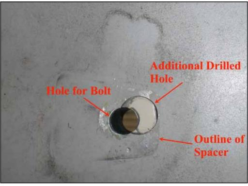
Photo No. 2: Drilled Holes in Skin
