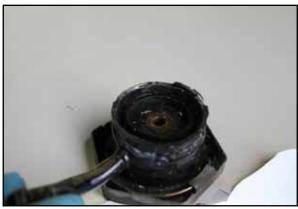
Photo No. 3: Vent cap with failed seal
