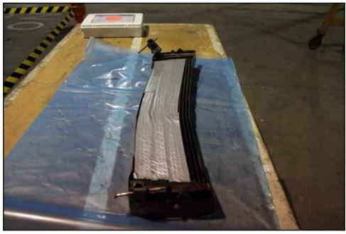
Photo No. 1: Radiator showing the taped upper surface
