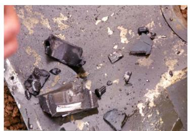
Fragments from the front main bearing housing and No.1 connecting rod big end as found on lower engine cowling.
