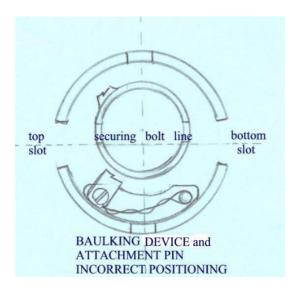
The technicians who removed and replaced the nose gear leg said that they reassembled the strut, attachment pin, baulking device and greasing plug in the way that they found it.
