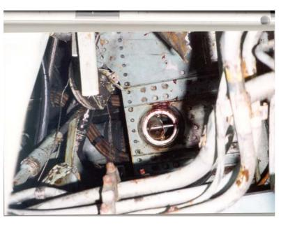
Securing Bolt in Baulking Device as found by investigators
