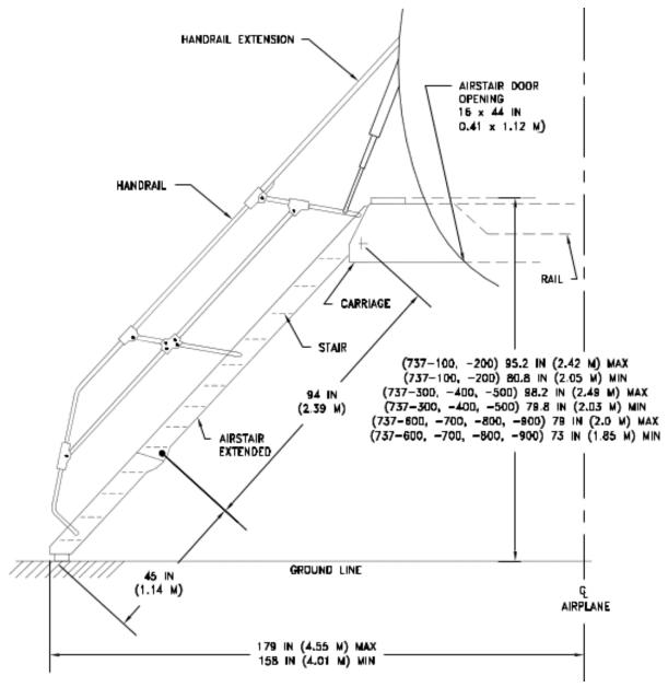
Figure 1: Dimensions of the stairs on the Boeing 737 aircraft
