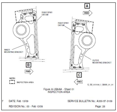
Figure No. 3: Original SB Diagram showing incorrect bracket pair
