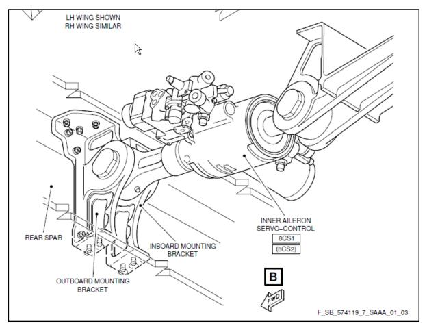
Figure No. 2: Engineering schematic of the assembly (LH Wing)
