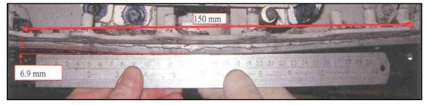
Photo No. 2: Deformation of lower wing skin, RH wing
