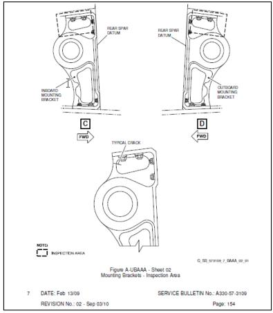
Figure No. 4: Revised SB diagram showing correct bracket pair
