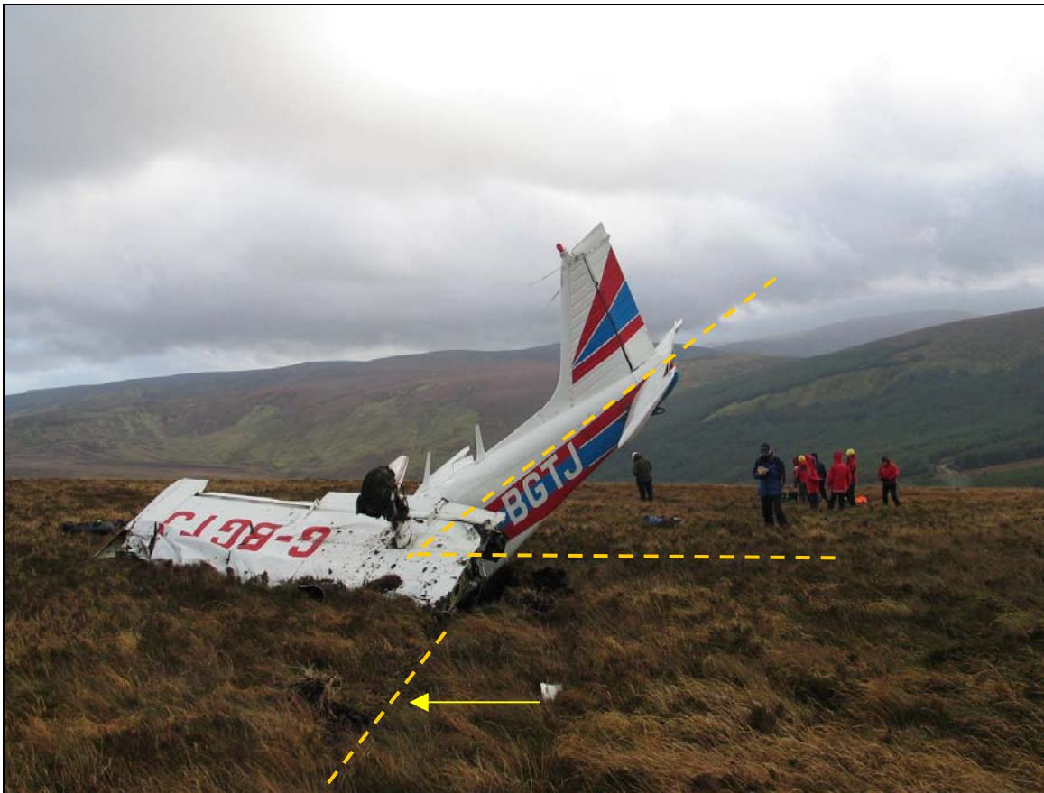
Photo No. 1: Wreckage impact angle and initial port wing impact (indicated by arrow)
