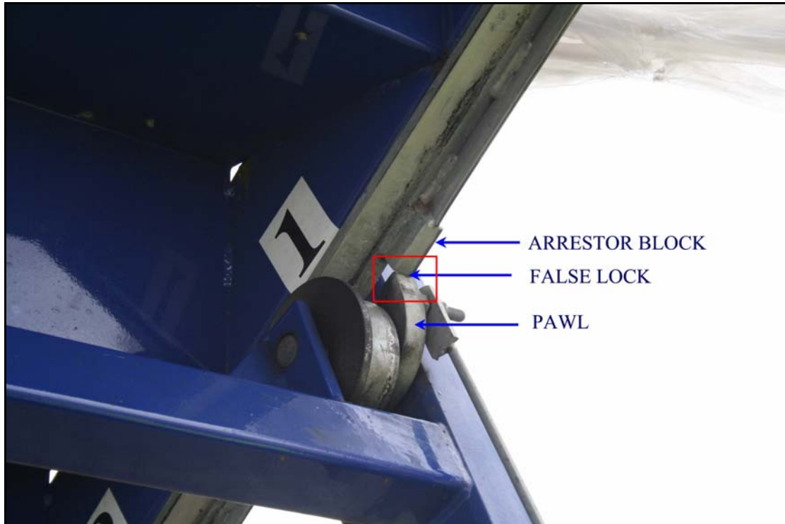
Photo No. 1: False lock configuration
