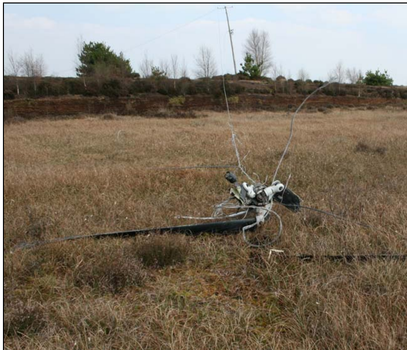
Photo No. 3: Detached Main Rotor, transmission pole is visible in the background
