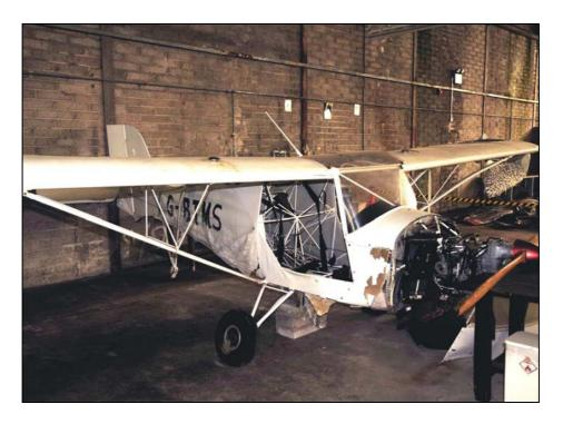
Photo No. 2: General view of wreckage with doors and seat removed
