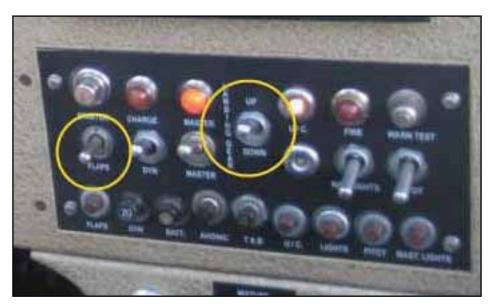
Photo No. 2: Centre instrument panel of El-BMF showing location of flaps and landing gear selector switches. (M. Nixon, 2009)
