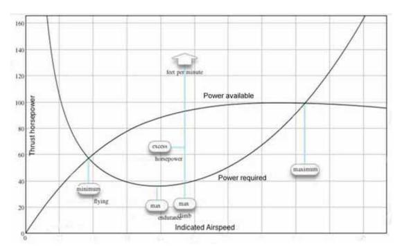
Figure No. 1: Illustration of power available and power required (total drag) curves (Benchmark)
