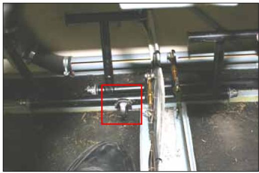
Photo No. 1: Fractured pedal assembly in-situ
