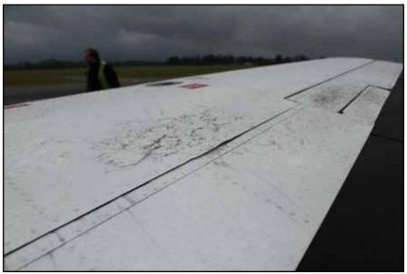
Photo No. 2: Damage to the wing upper surface
