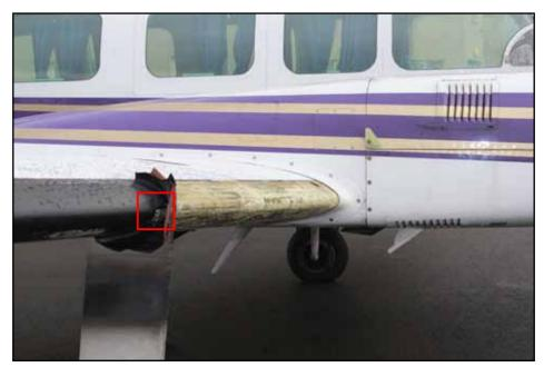
Photo No. 1: De-ice boot peeling (stall warning vane marked in red)
