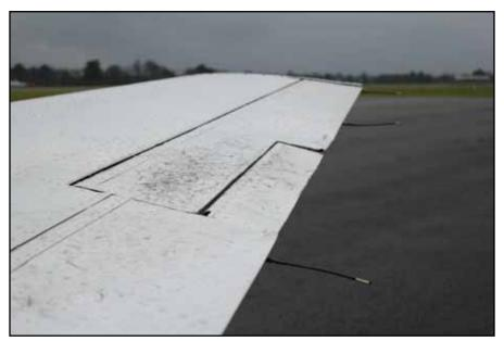
Photo No. 3: Damage to the starboard aileron
