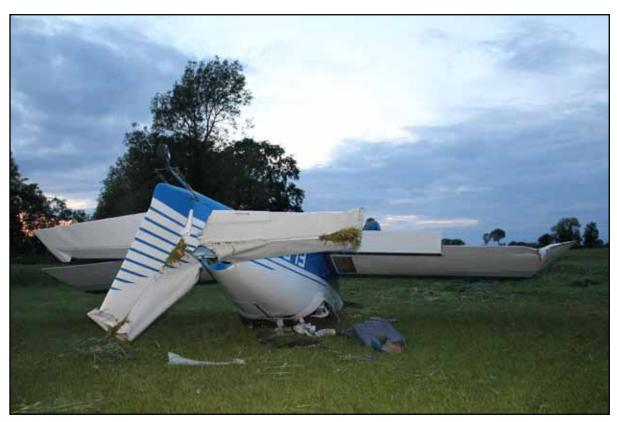
Photo No. 1: The inverted aircraft and smashed canopy.
