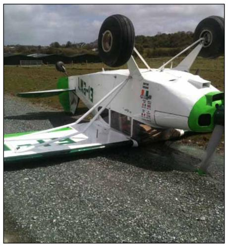
Photo No. 1: Aircraft in final inverted position (Pilot's Photo).
