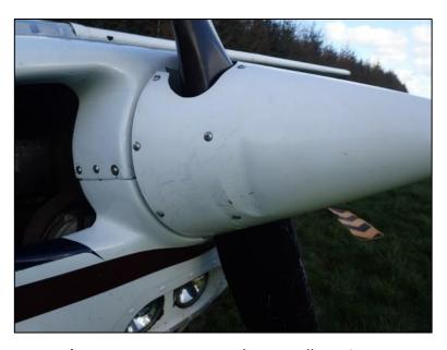
Photo No. 5: Damage to the propeller spinner
