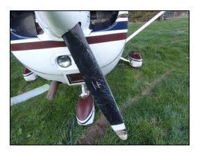
Photo No. 3 (left) and Photo No. 4 (right): Damage to right wing tip and propeller blade
