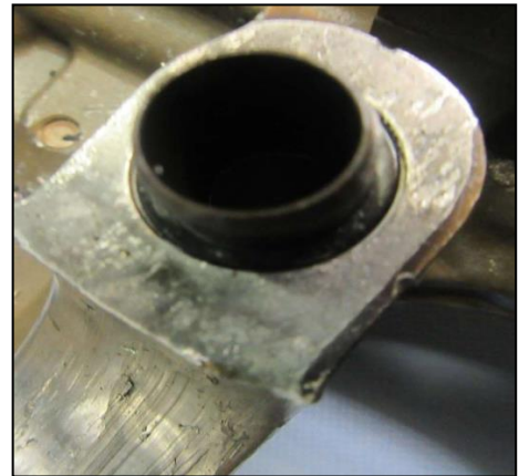
Photo No. 14: Fretting of the No. 2 main bearing crankcase saddle and heavy wear to the bearing bore material
