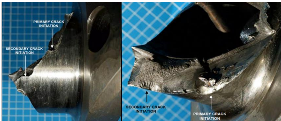
Figure No. A1: Crack #1 initiation site on MJ #2
