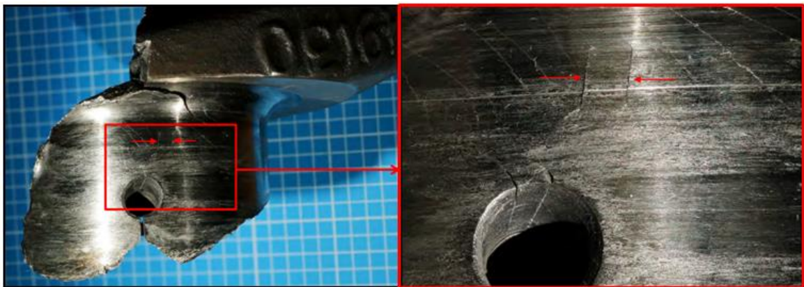
Figure No. A6: Close-up of longitudinal cracks on surface of MJ #2
