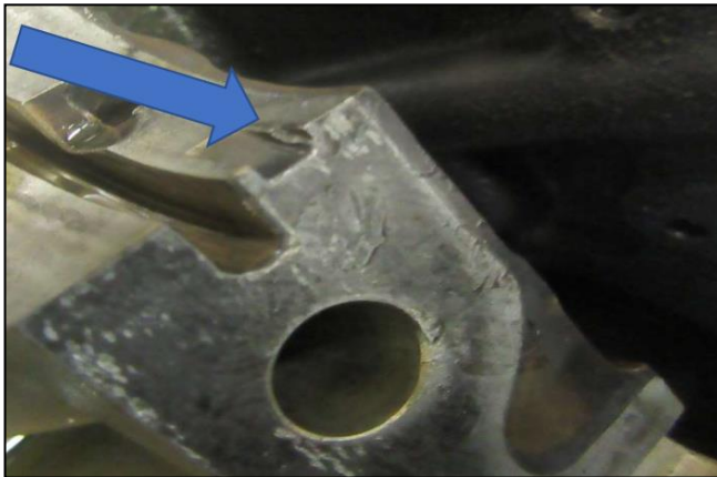
Photo No. 13: Fretting and tang slot wear to the No. 1 main bearing crankcase saddle
