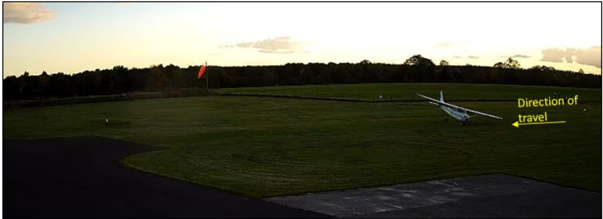
Figure No. 1: Sideways skid of aircraft coming to the end of grass surface
