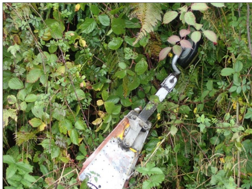
Photo No. 12: Tailwheel assembly as located within the hedgerow
