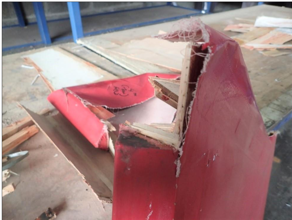
Photo No. 15: Fractured and separated upper portion of the rudder
