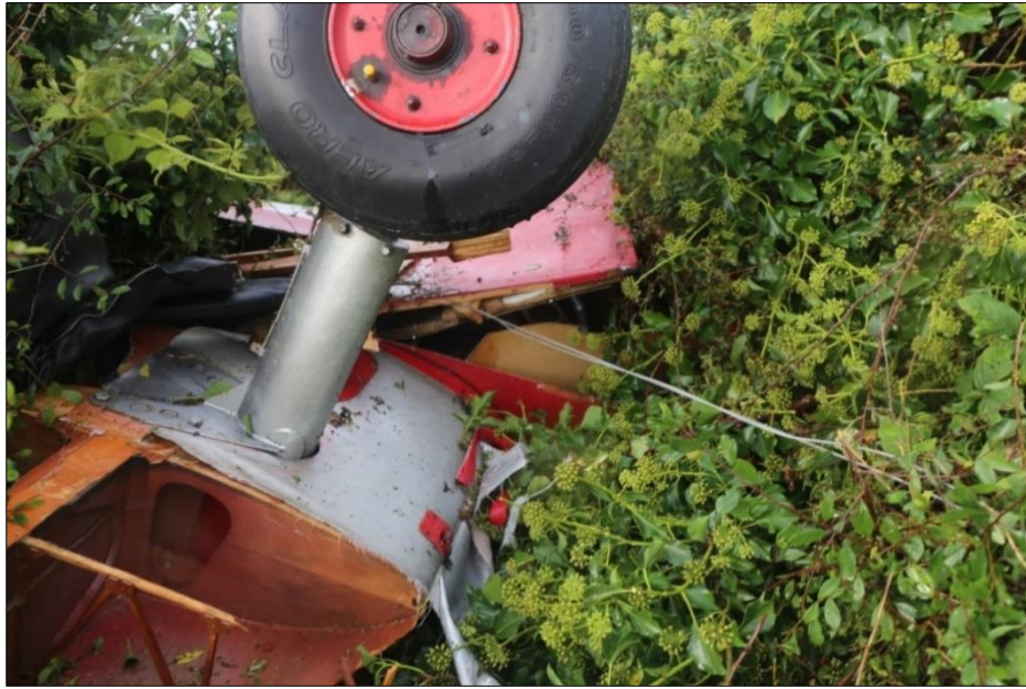
Photo No. 4: Inboard section of left wing (inverted) that remained attached
