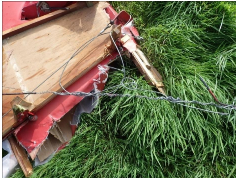
Photo No. 6: Control cables from the aircraft tail still attached to the main wreckage
