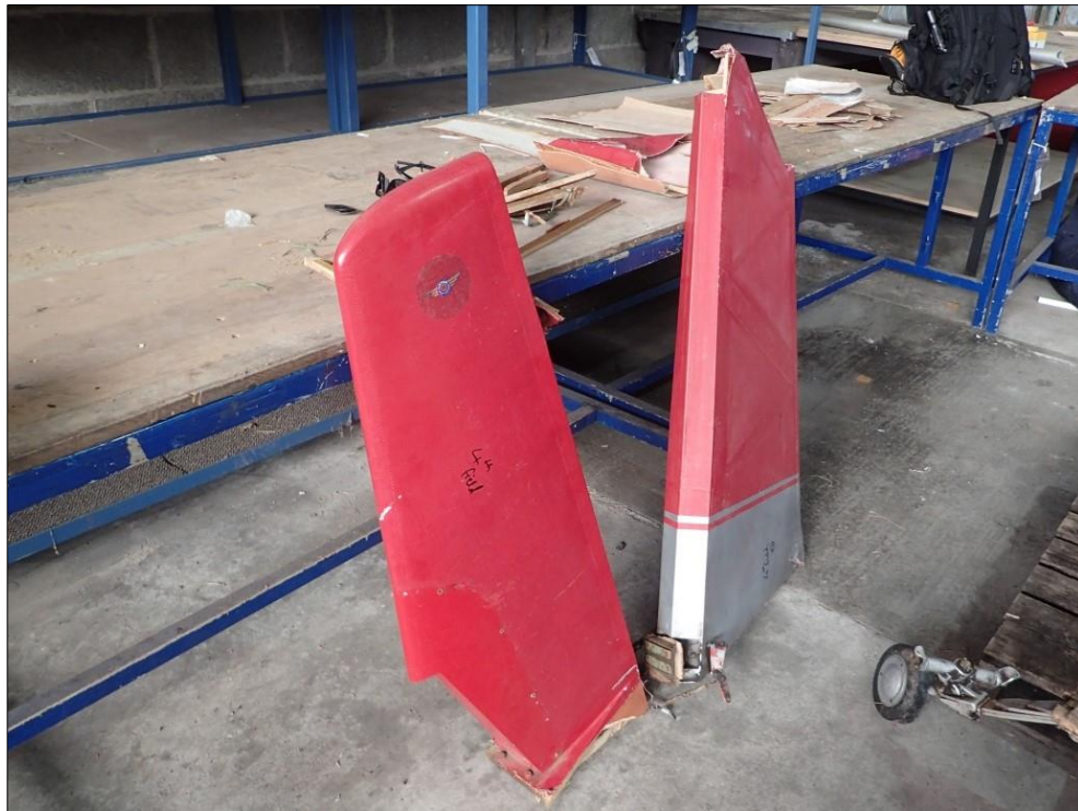
Photo No. 14: Vertical stabiliser (red) and rudder (red/silver)
