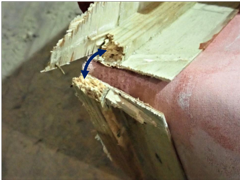
Photo No. 16: Fractured surfaces of the separated upper portion of the rudder
