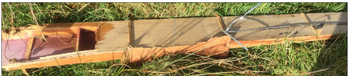
Photo No. 7: Separated front spar from the left wing
